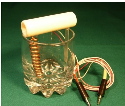
Cooper-Silver electrochemical cell
